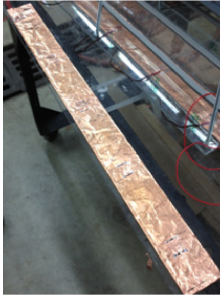
Figure 4.2: Copper sheet wrapped on heating element used for testing.
